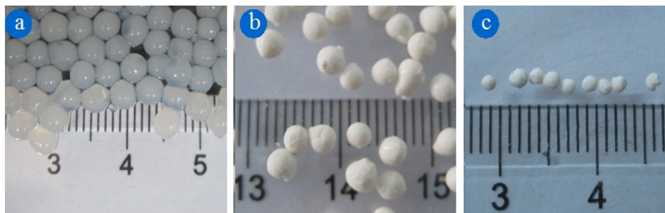
Fig. 2. Optical photographs of CS-PVA beads (a), UTS (b) and CTS-500 (c).
